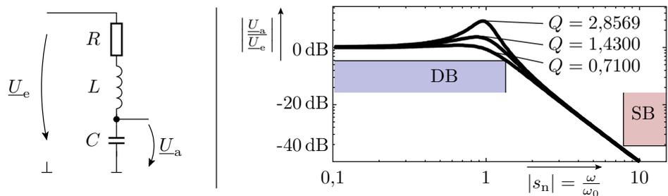
$$\frac{U_a}{U_e} = \frac{1}{R + j \cdot \omega \cdot L + \frac{1}{j \cdot \omega \cdot C}} = \frac{1}{1 + \frac{j \cdot \omega}{Q \cdot \omega_0} - \left(\frac{\omega}{\omega_0}\right)^2}$$
