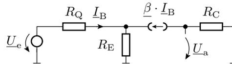
$$\begin{aligned} \underline{U}_e &= (R_Q + R_E \cdot (1 + \underline{\beta})) \cdot \underline{I}_B \\ \underline{U}_a &= -R_C \cdot \underline{\beta} \cdot \underline{I}_B \\ &= -\frac{R_C \cdot \underline{\beta} \cdot \underline{U}_e}{R_Q + R_E \cdot (1 + \underline{\beta})} \\ &= -\frac{R_C \cdot \underline{U}_Q}{(R_Q + R_E) \cdot \frac{1}{\underline{\beta}} + R_E} \end{aligned}$$
