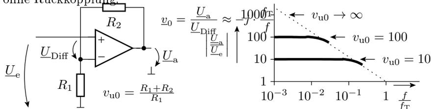
$$\underline{U}_a = \underline{v}_0 \cdot \left( \underline{U}_e - \frac{\underline{U}_a}{v_{u0}} \right) \quad \text{mit } v_{u0} = \frac{R_1 + R_2}{R_1}; \quad \underline{v}_0 \approx -j \cdot \frac{f_T}{f}$$
