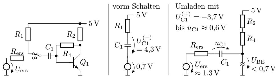
$$\tau = C_1 \cdot (R_{ers} + R_2 + R_4)$$
