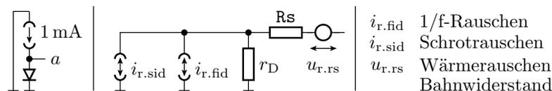
$I = 1 \text{ mA}$ ,  $f_u = 10 \text{ Hz}$ ;  $f_o = 10 \text{ MHz} \approx \Delta f$ ,  $R_S = 0,568 \Omega$ ;  $r_D = \frac{dU_D}{dI_D}$  für  $I_D = 1 \text{ mA}$  laut Simulation  $46 \Omega$ ;  $Kf = 1,2$ ;  $Af = 10^{-15} \text{ A}^{0,2}$ :
