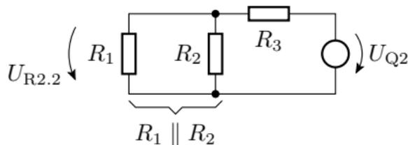
$$U_{R2} = U_{R2.1} + U_{R2.2} = U_{Q1} \cdot \frac{R_2 \parallel R_3}{(R_2 \parallel R_3) + R_1} + U_{Q2} \cdot \frac{R_1 \parallel R_2}{(R_1 \parallel R_2) + R_3}$$
