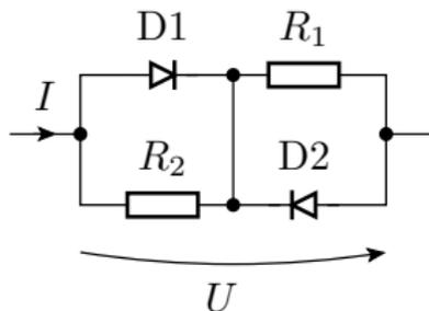
$$R_1 = R_2 = 1 \text{ k}\Omega$$
