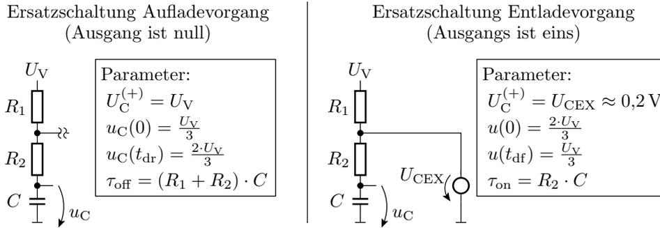
$$u_C(t_{on}) = \frac{1}{3} \cdot U_V = U_{CEX} - \left( U_{CEX} - \frac{2}{3} \cdot U_V \right) \cdot e^{-\frac{t_{on}}{R_2 \cdot C}}$$
