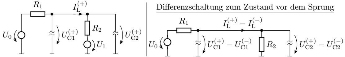
$$U_{C1}^{(+)} - U_{C1}^{(-)} = U_{C2}^{(+)} - U_{C2}^{(-)} = U_0 \cdot \frac{R_2}{R_1 + R_2}$$
