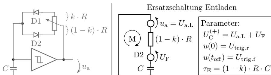
$$t_{\text{off}} = (1 - k) \cdot R \cdot C \cdot \ln \left( \frac{U_{\text{a.L}} + U_{\text{F}} - U_{\text{trig.r}}}{U_{\text{a.L}} + U_{\text{F}} - U_{\text{trig.f}}} \right)$$
