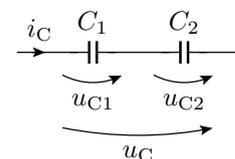
$$\begin{aligned} u_C &= u_{C,1} + u_{C,2} \\ &= \frac{1}{C_1} \cdot \int_{t_0}^t i_C(\tau) \cdot d\tau + \frac{1}{C_2} \cdot \int_{t_0}^t i_C(\tau) \cdot d\tau + u_{C,1}(t_0) + u_{C,2}(t_0) \\ &= \left( \frac{1}{C_1} + \frac{1}{C_2} \right) \cdot \int_{t_0}^t i_C(\tau) \cdot d\tau + u_{C,1}(t_0) + u_{C,2}(t_0) \end{aligned}$$
