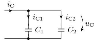
$$i_C = C \cdot \frac{du_C}{dt} = i_{C.1} + i_{C.2} = C_1 \cdot \frac{du_C}{dt} + C_2 \cdot \frac{du_C}{dt}$$
