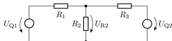
$$U_{R2} = \underbrace{\frac{R_2 \parallel R_3}{R_1 + (R_2 \parallel R_3)}}_{U_{R2.1}} \cdot U_{Q1} + \underbrace{\frac{R_1 \parallel R_2}{R_3 + (R_1 \parallel R_2)}}_{U_{R2.2}} \cdot U_{Q2}$$
