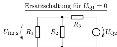
$$U_{R2.2} = \frac{R_1 \parallel R_2}{R_3 + (R_1 \parallel R_2)} \cdot U_{Q2}$$
