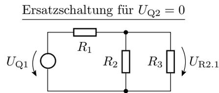
$$U_{R2.1} = \frac{R_2 \parallel R_3}{R_1 + (R_2 \parallel R_3)} \cdot U_{Q1}$$
