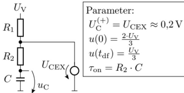
$$u_C(t_{on}) = \frac{1}{3} \cdot U_V = U_{CEX} - \left( U_{CEX} - \frac{2}{3} \cdot U_V \right) \cdot e^{-\frac{t_{on}}{R_2 \cdot C}}$$
