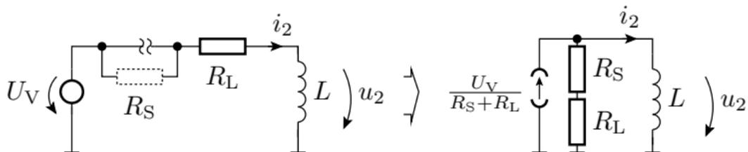
$$I_2^{(+)} = \lim_{R_S \rightarrow \infty} \left( \frac{U_V}{R_L + R_S} \right) = 0$$
