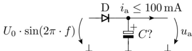
$$\left| \begin{array}{l} U_0 = 12 \text{ V} \\ \Delta U_{\text{a.rel}} \leq 5\% \\ f = 50 \text{ Hz} \end{array} \right.$$
