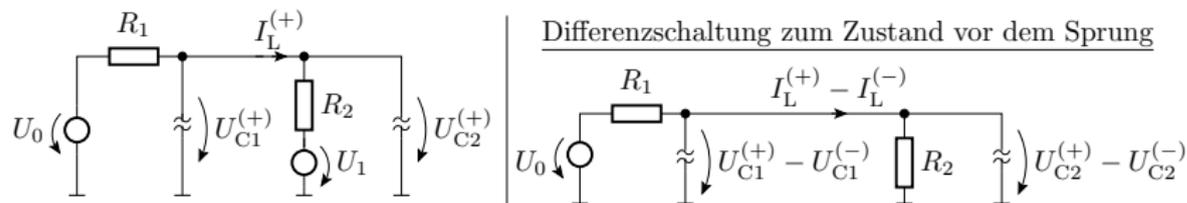
$$U_{C1}^{(+)} - U_{C1}^{(-)} = U_{C2}^{(+)} - U_{C2}^{(-)} = U_0 \cdot \frac{R_2}{R_1 + R_2}$$
