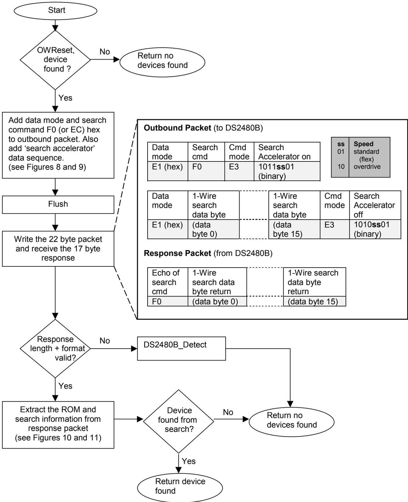
The state of the 1-Wire search must be maintained between searches to find subsequent devices. The terms representing the search state are presented in Table 5 and coincide with the terms used in Application Note 187, *The 1-Wire Search Algorithm*.
