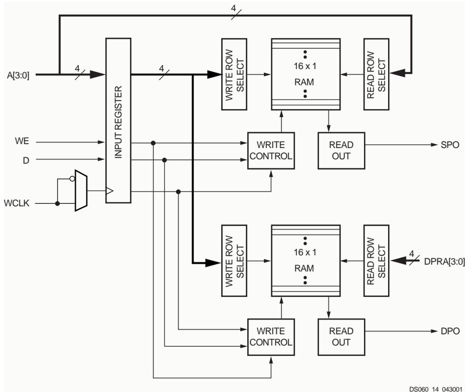
Figure 14: Logic Diagram for the Dual-Port RAM
