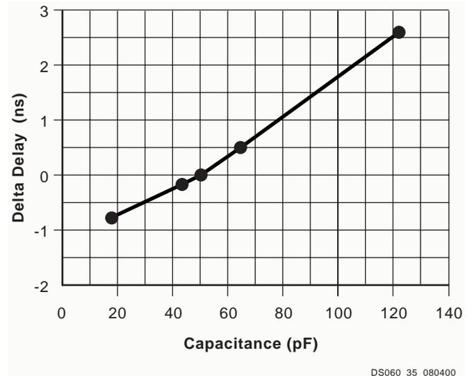
Figure 34: Delay Factor at Various Capacitive Loads
