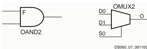
Figure 7: AND and MUX Symbols in Spartan-XL IOB
