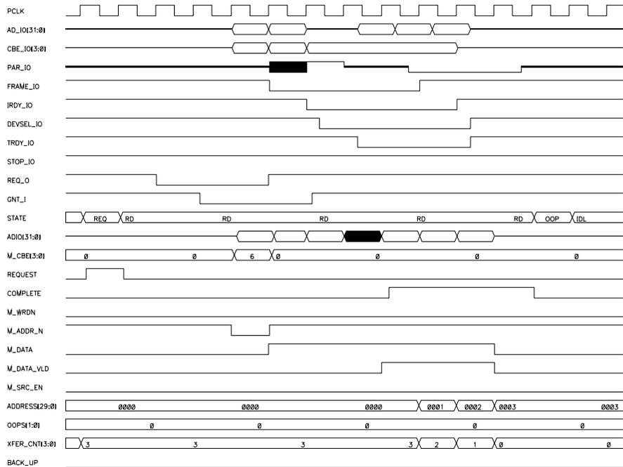
**Figure 14-5 Burst Read Transaction with Normal Termination**
