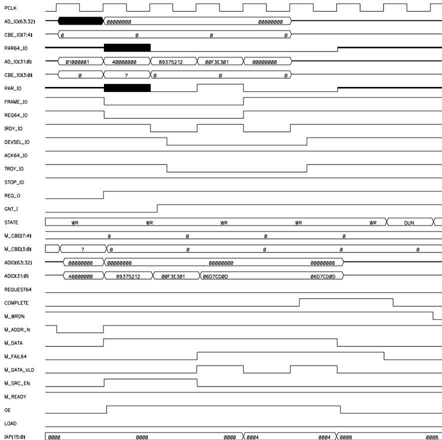
**Figure 15-5 32-bit Target Responds to 64-bit Write**
