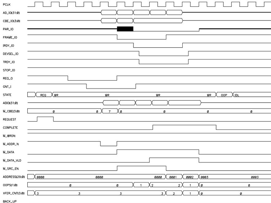
**Figure 14-6 Burst Write Transaction with Normal Termination**
