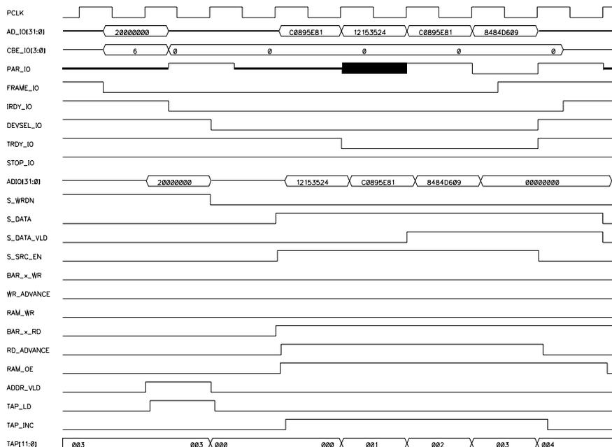
**Figure 8-2 Target Burst Read Transaction**
