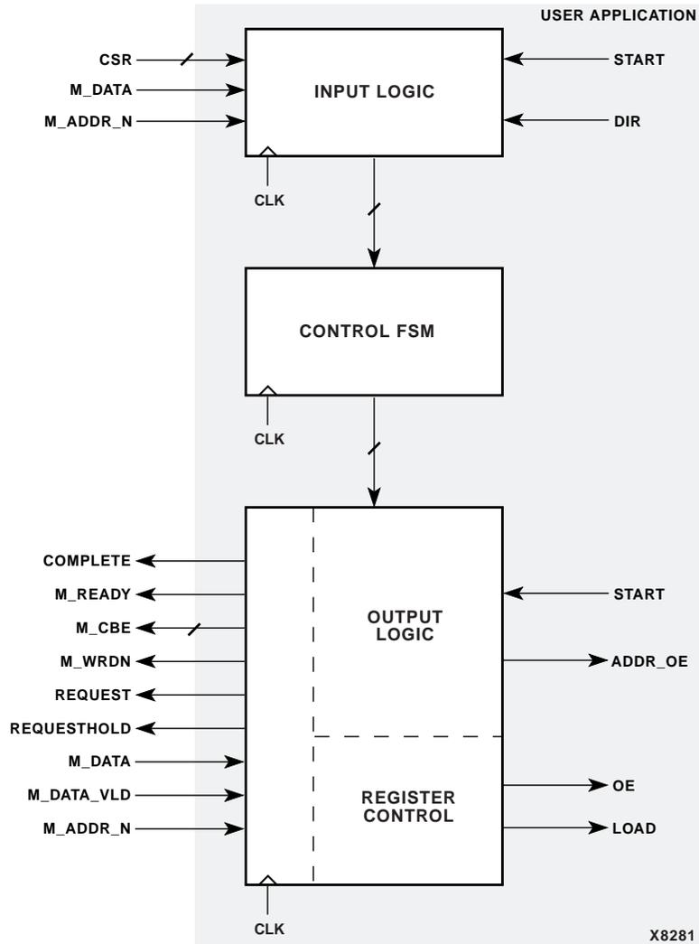
**Figure 12-2 Initiator Control Block Diagram**
