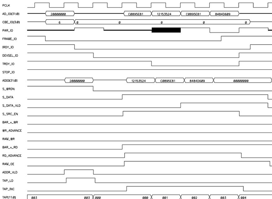
**Figure 8-2 Target Burst Read Transaction**
