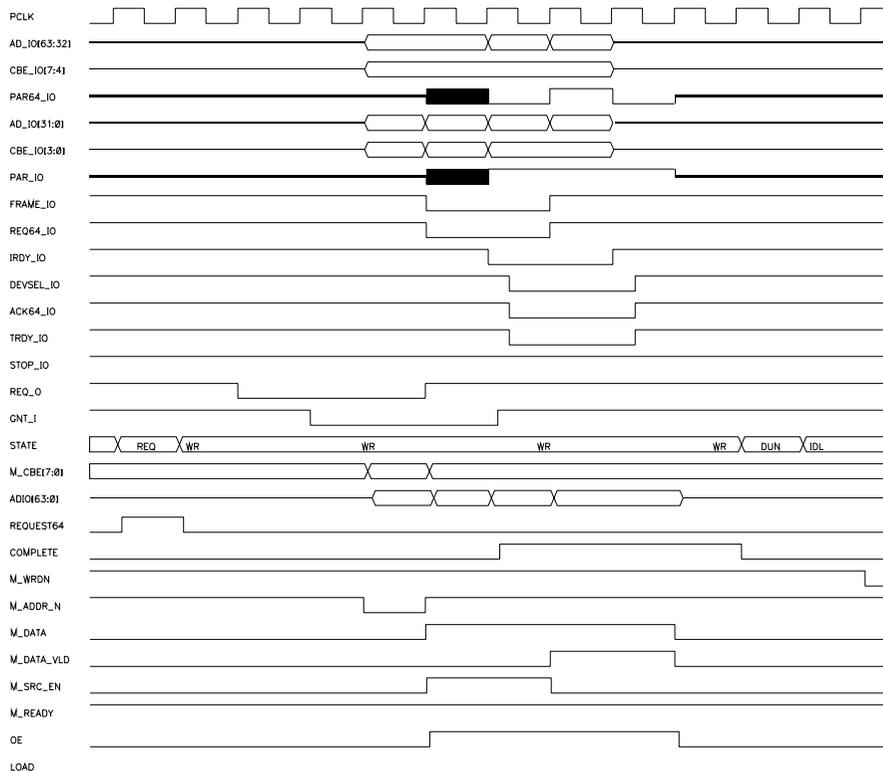
**Figure 15-2 Two QWORD Initiator Write Transfer**
