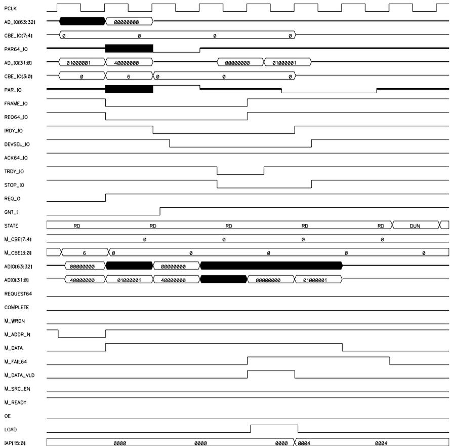
**Figure 15-4 32-bit Target Disconnects with Data on Read**
