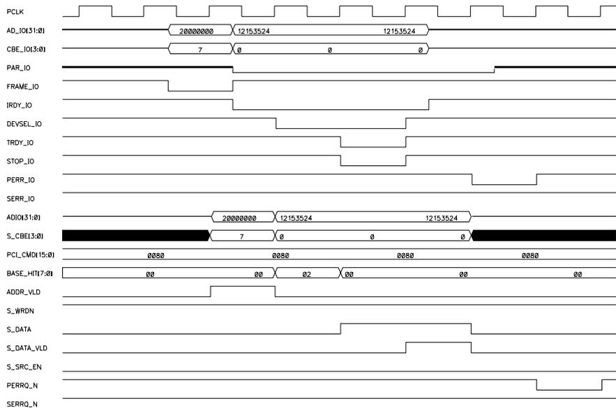
**Figure 17-3 Target Write with Data Parity Error**
