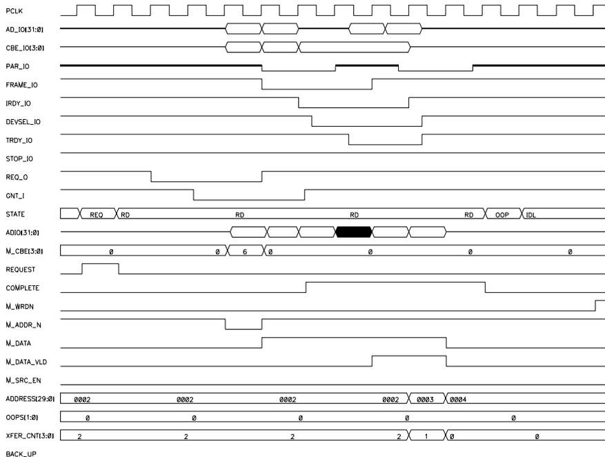
**Figure 14-8 Burst Read Continues after Target Disconnect**
