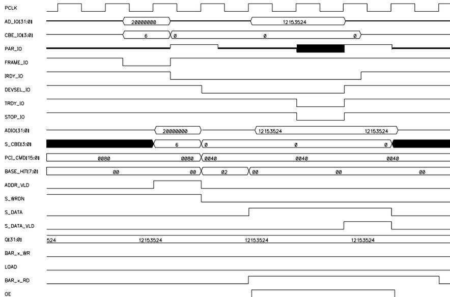
Figure 6-3 Target Read Transaction
