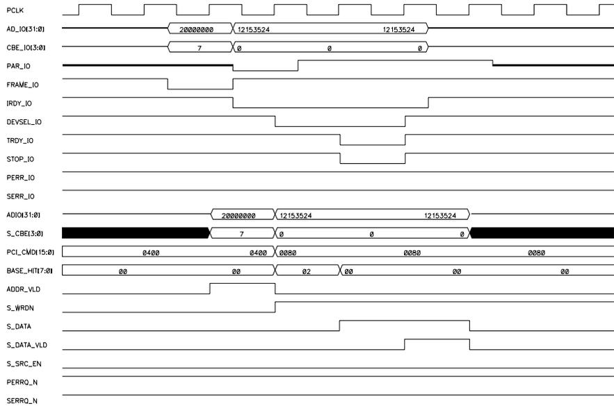
**Figure 17-1 Target Write with no Parity Errors**
