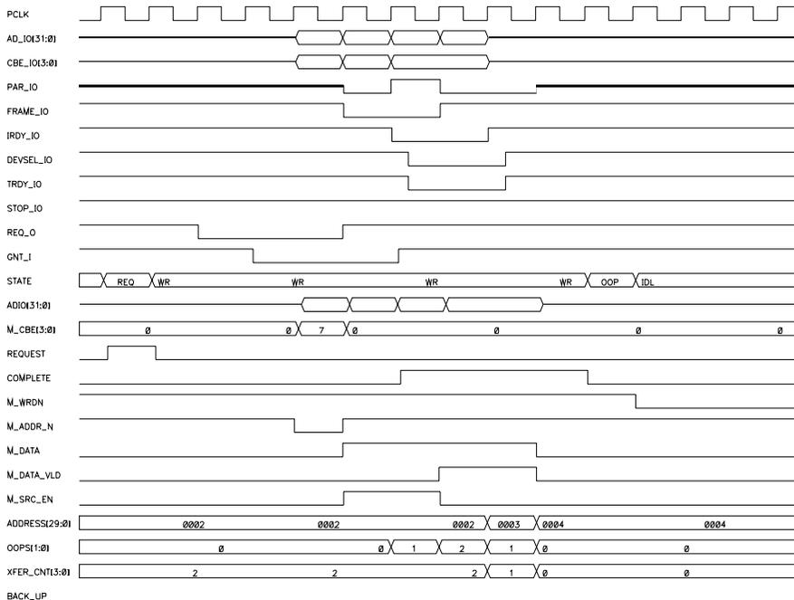
**Figure 14-10 Burst Write Continues after Target Disconnect**
