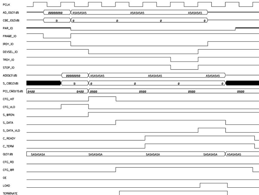
**Figure 16-4 Configuration Write with Wait States**
