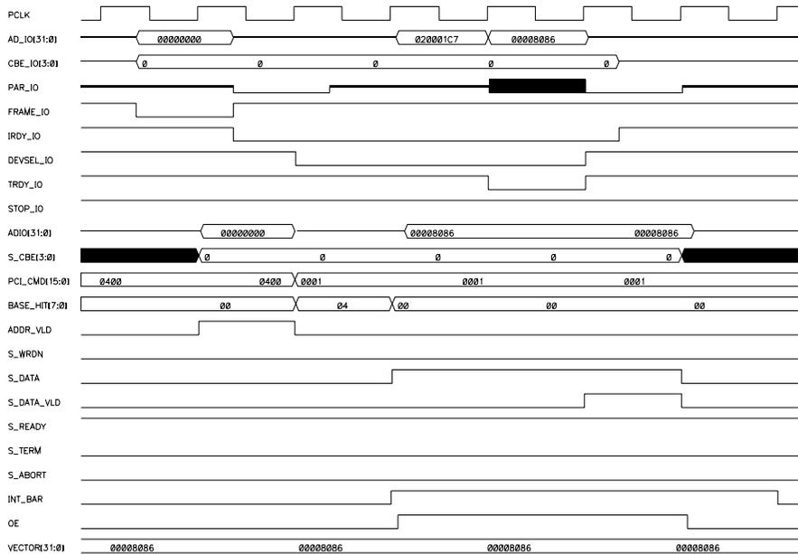
Figure 16-1 Target Accepts Interrupt Acknowledge Cycle
