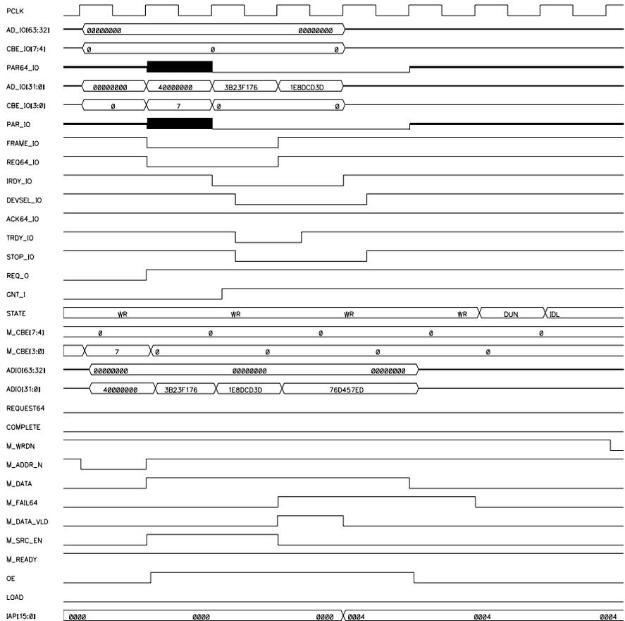
**Figure 15-6 32-bit Target Disconnects with Data on Write**
