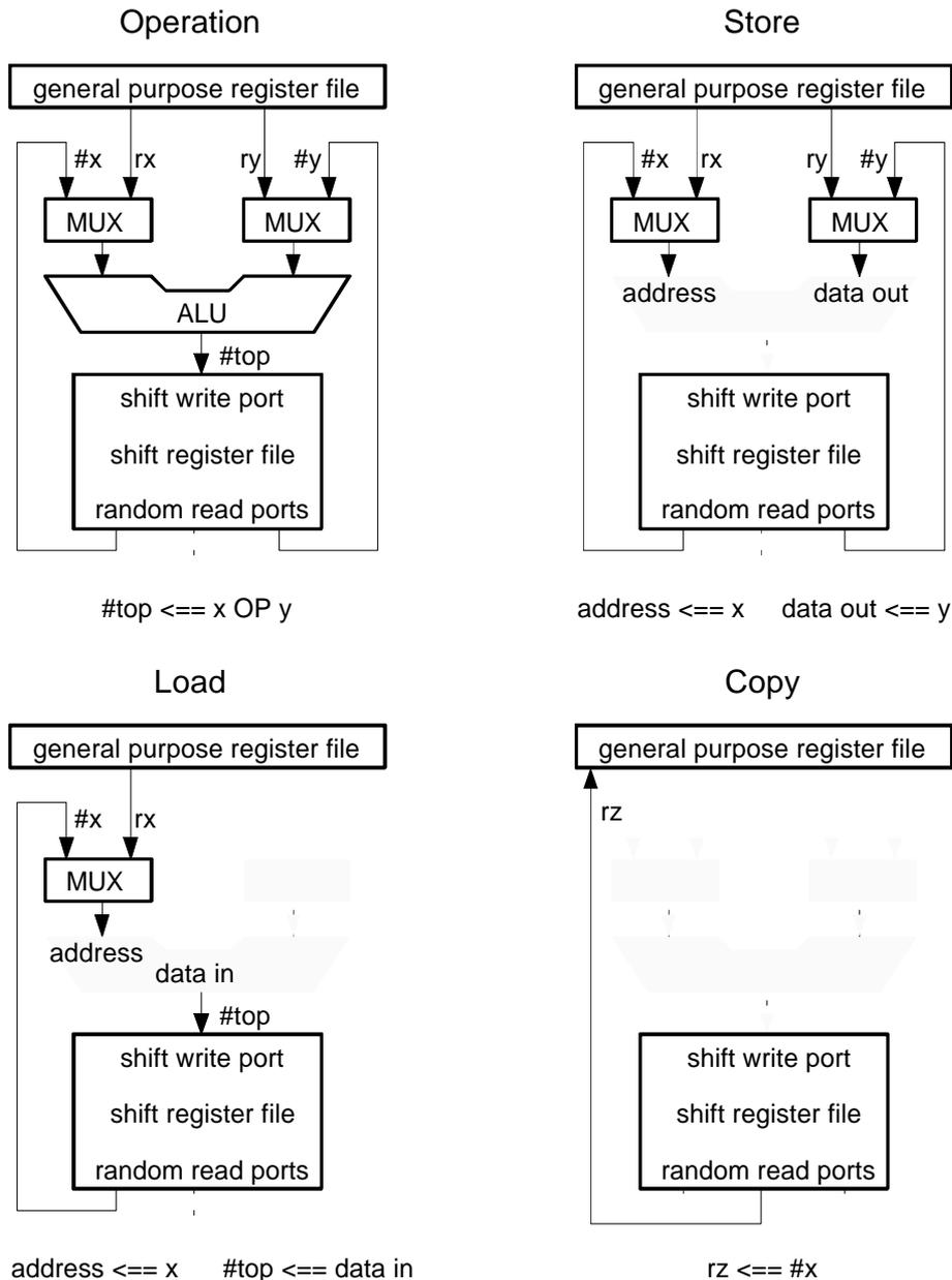
Figure 5: Data path for ALU operation, load, store, and copy
