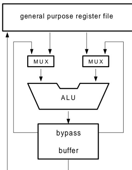
Figure 3: Conventional ALU with bypass buffer
