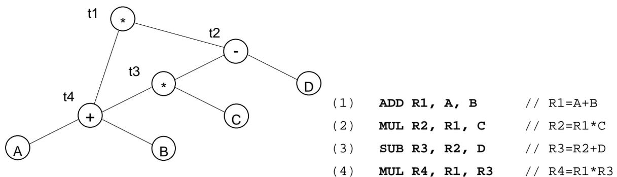
Figure 1: Directed acyclic graph and RISC program to calculate  $(A + B) * ((A + B) * C - D)$
