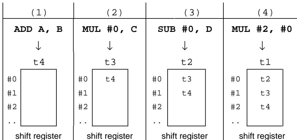
Figure 2: Passing temporaries via shift register
