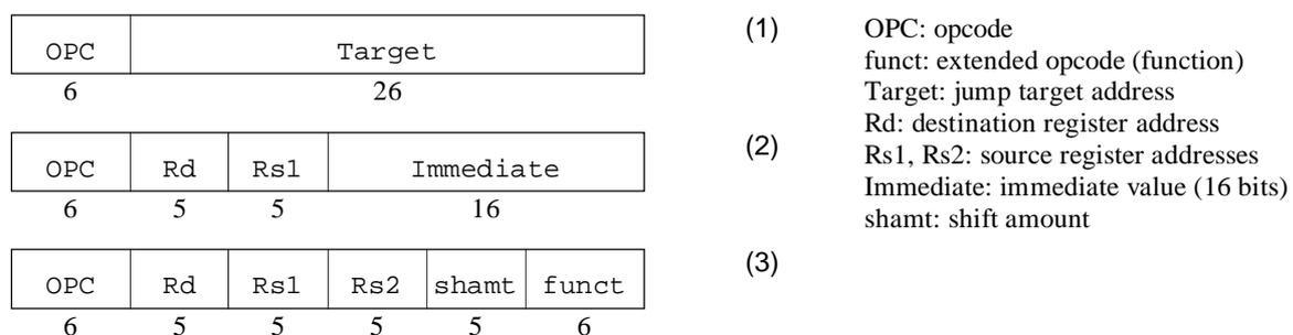
Figure 7: Instruction formats of the MIPS processor [3]
