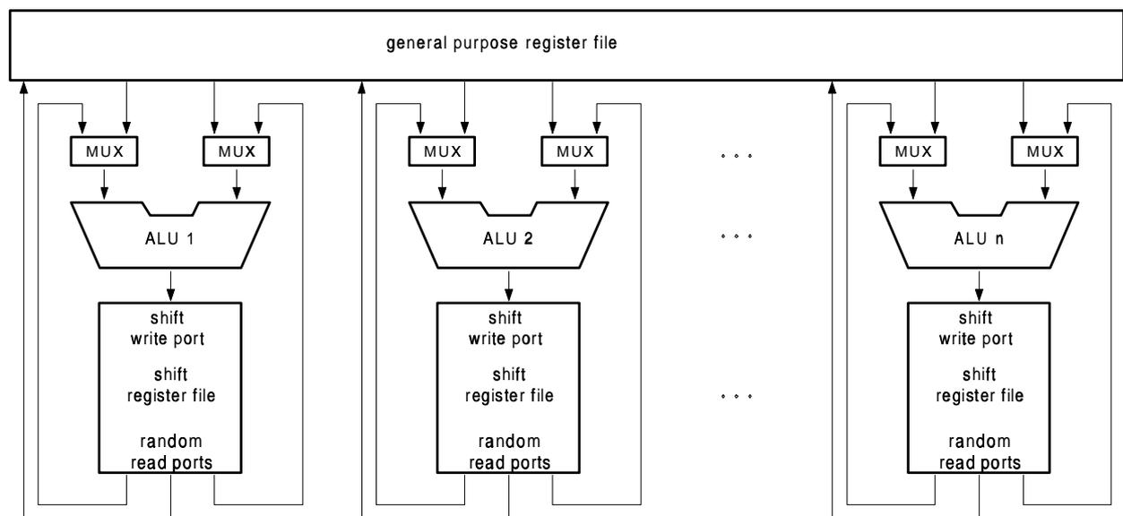
Figure 6: Data path of a VLIW- or a superscalar processor using shift registers for the results
