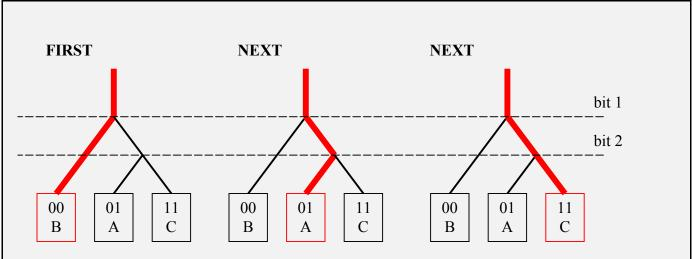
**Note:** Each branching at a bit level denotes a 'discrepancy' where the both the bit and complement-bit return '0'.
