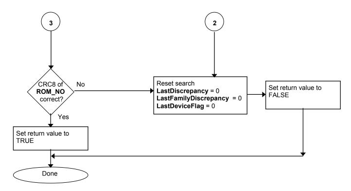
There are two basic types of operations that can be performed by using the search algorithm by manipulating the LastDiscrepancy, LastFamilyDiscrepancy, LastDeviceFlag, and ROM\_NO register values (see Table 4). These operations concern basic discovery of the ROM numbers of 1-Wire devices.
