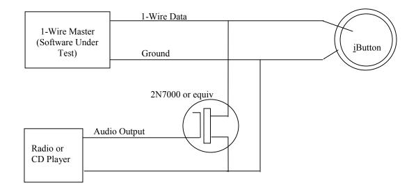
(Various improvements could be made to this test circuit, but that is beyond the scope of this document. The bus should be intermittently shorted but not driven to levels that violate the component maximum ratings.)
