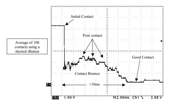
The waveform above demonstrates that the electrical contact between the reader probe and the <u>i</u>Button does not stabilize until as long as 10ms or more after the initial contact is made. More than 40% of the <u>i</u>Button arrivals in this test had no stable connection even 6ms after the initial contact.
