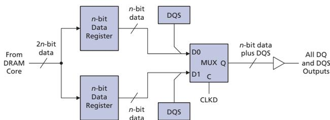
To the user, from a high-level view, 2n-prefetch means that data accesses occur in pairs; i.e., a single read access fetches two data words; and for a single write access, two data words (and/or data mask bits) must be provided. This affects both the minimum burst size and nonminimum burst interruptions. The minimum burst size of a 2n-prefetch architecture is two external data transfers.
