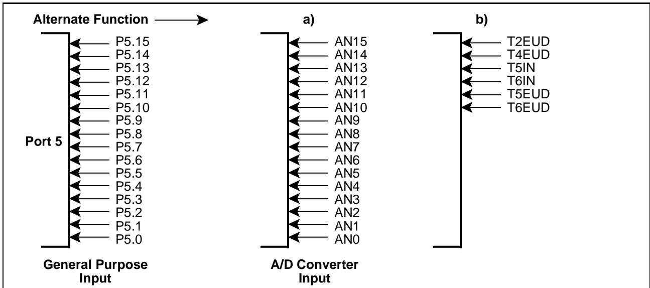
Figure 6-15 Port 5 IO and Alternate Functions
