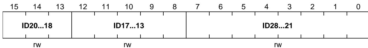
**Lower Mask of Last Message (EF0E<sub>H</sub>)      XReg      Reset Value: UUUU<sub>H</sub>**
