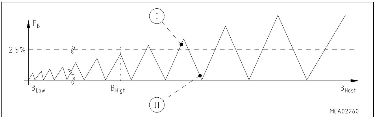
**Figure 13-3**Baudrate deviation between host and C167
