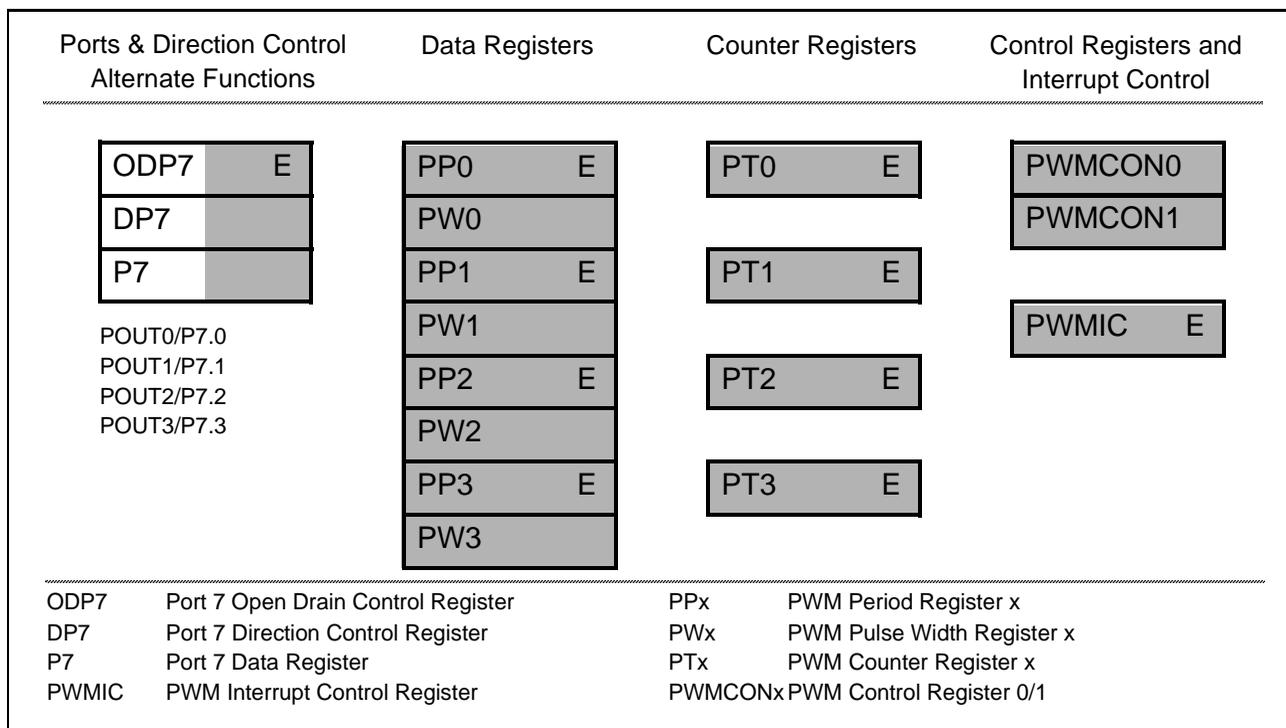
Figure 15-1 SFRs and Port Pins Associated with the PWM Module
