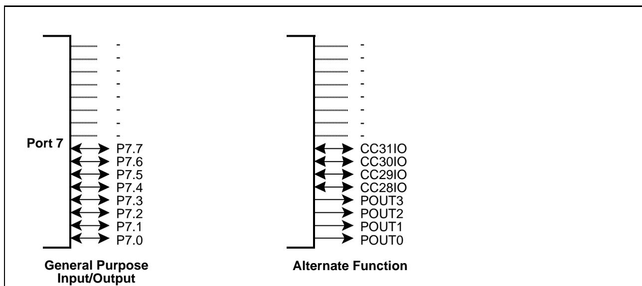
**Figure 6-20** Port 7 IO and Alternate Functions
