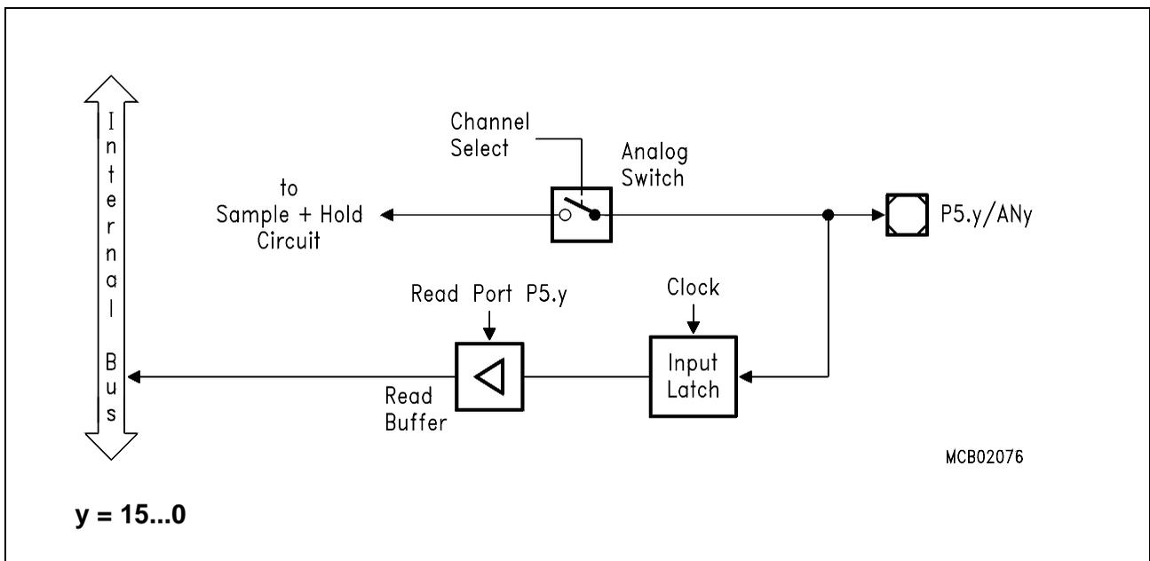
Figure 6-16 Block Diagram of a Port 5 Pin
