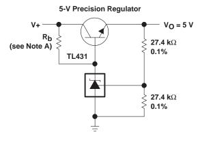
NOTE A: R<sub>b</sub> should provide cathode current  $\geq$  1 mA to the TL431.
