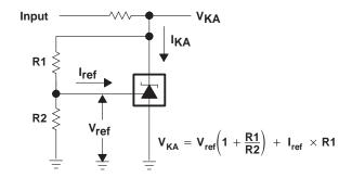
Figure 3. Test Circuit for  $V_{KA} > V_{ref}$
