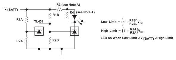
NOTE A: R3 and R4 are selected to provide the desired LED intensity and cathode current ≥ 1 mA to the TL431 at the available V<sub>I(BATT)</sub>.
