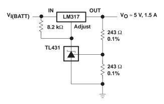
Figure 23. Precision 5-V 1.5-A Regulator
