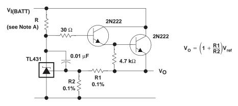
NOTE A: R should provide cathode current ≥ 1 mA to the TL431 at minimum V<sub>I</sub>(BATT).
