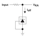
Figure 4. Test Circuit for Ioff
