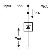
Figure 2. Test Circuit for  $V_{KA} = V_{ref}$
