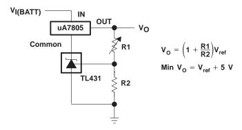
Figure 20. Output Control of a Three-Terminal Fixed Regulator
