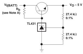
NOTE A:  $R_b$  should provide cathode current  $\geq$  1-mA to the TL431.
