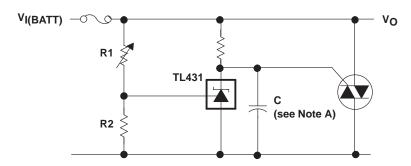
NOTE A: Refer to the stability boundary conditions in Figure 16 to determine allowable values for C.
