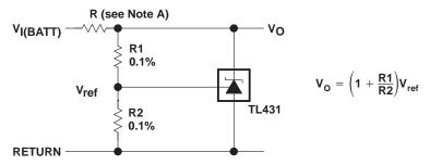
NOTE A: R should provide cathode current ≥ 1 mA to the TL431 at minimum V<sub>I(BATT)</sub>.
