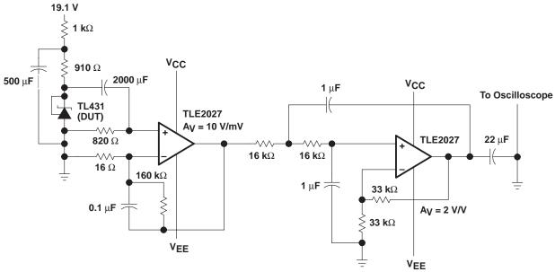
Figure 12. Test Circuit for Equivalent-Input Noise Voltage
