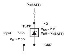
Figure 18. Single-Supply Comparator With Temperature-Compensated Threshold
