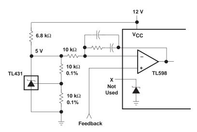
Figure 25. PWM Converter With Reference
