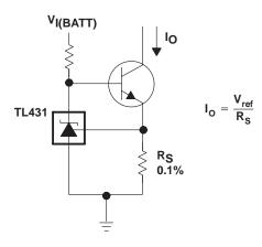
Figure 29. Precision Constant-Current Sink
