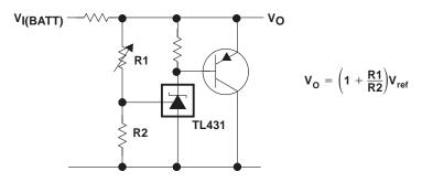
Figure 21. High-Current Shunt Regulator
