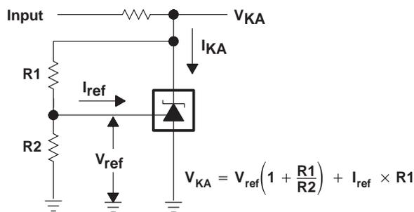
Figure 3. Test Circuit for  $V_{\text{KA}} > V_{\text{ref}}$
