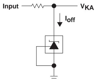
Figure 4. Test Circuit for  $I_{\text{off}}$
