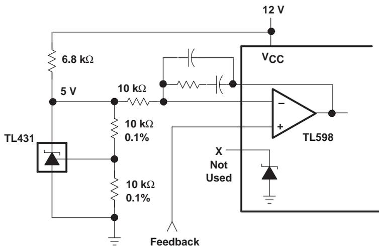
Figure 25. PWM Converter With Reference
