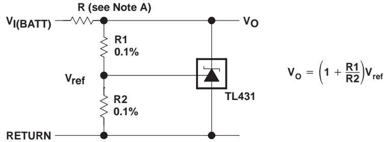
NOTE A: R should provide cathode current  $\geq 1$  mA to the TL431 at minimum  $V_{I(BATT)}$ .
