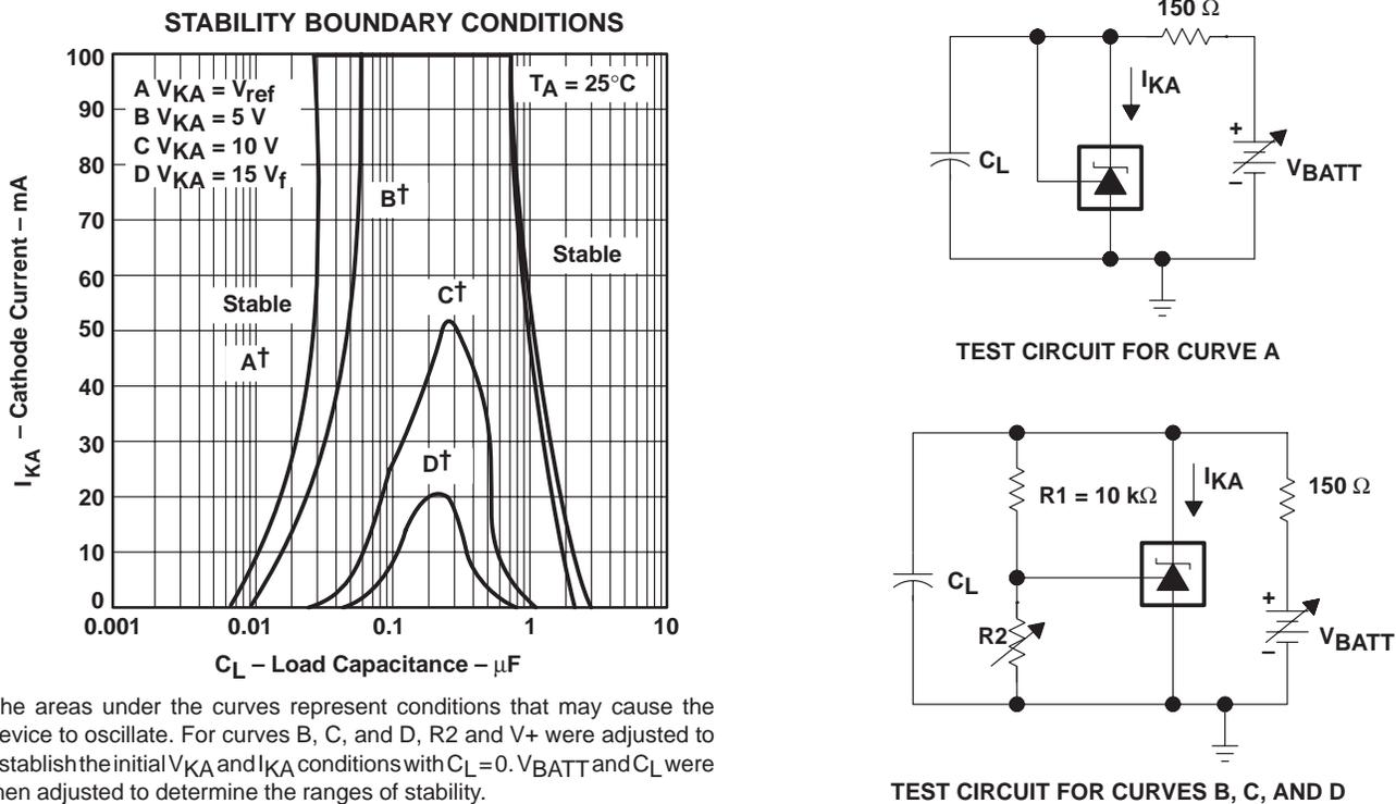
† The areas under the curves represent conditions that may cause the device to oscillate. For curves B, C, and D, R2 and V+ were adjusted to establish the initial  $V_{KA}$  and  $I_{KA}$  conditions with  $C_L = 0$ .  $V_{BATT}$  and  $C_L$  were then adjusted to determine the ranges of stability.
