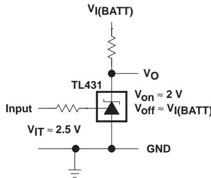
Figure 18. Single-Supply Comparator With Temperature-Compensated Threshold
