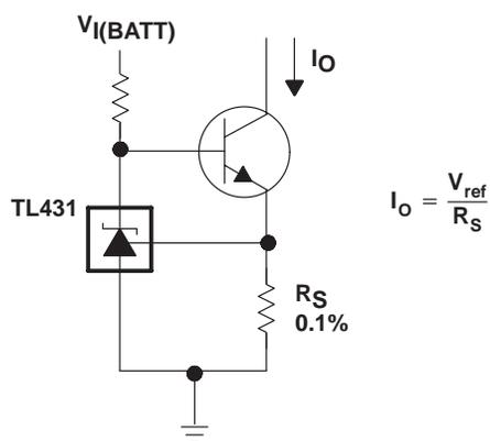
Figure 29. Precision Constant-Current Sink
