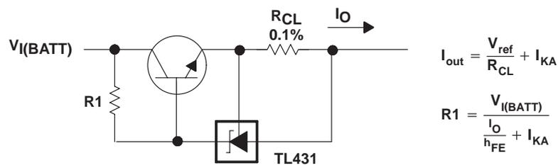
Figure 28. Precision Current Limiter
