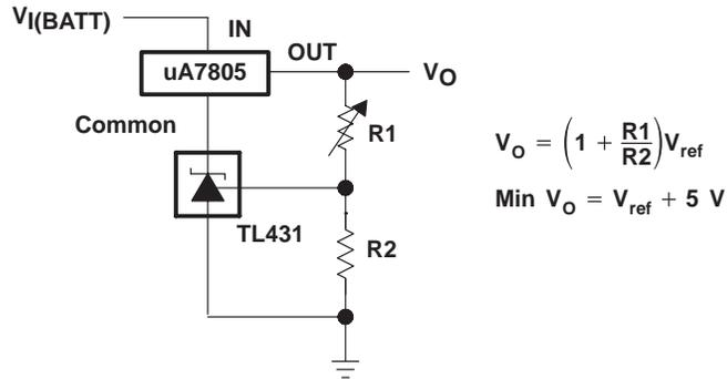
Figure 20. Output Control of a Three-Terminal Fixed Regulator
