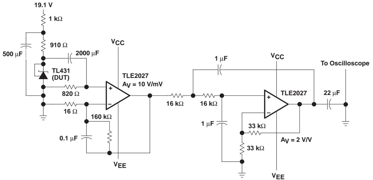
Figure 12. Test Circuit for Equivalent-Input Noise Voltage
