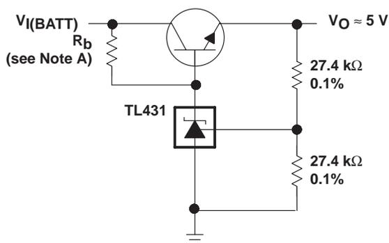
NOTE A:  $R_b$  should provide cathode current  $\geq 1\text{-mA}$  to the TL431.
