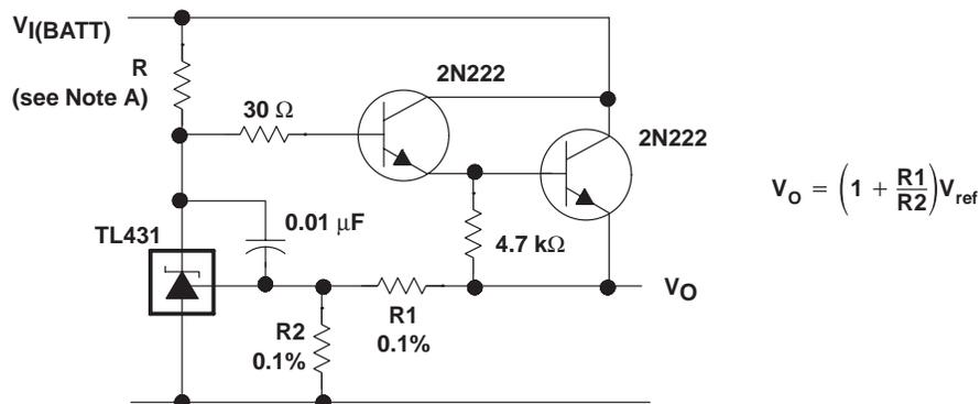
NOTE A: R should provide cathode current  $\geq 1$  mA to the TL431 at minimum  $V_{I(BATT)}$ .
