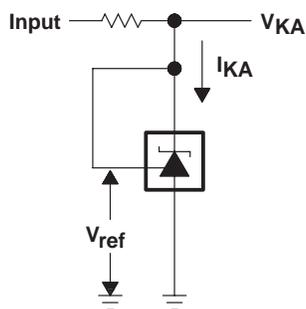
Figure 2. Test Circuit for  $V_{\text{KA}} = V_{\text{ref}}$
