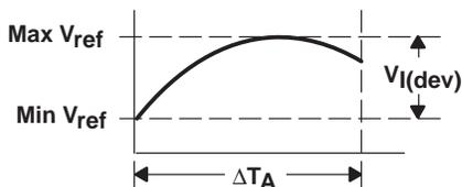
where  $\Delta T_A$  is the rated operating free-air temperature range of the device.
