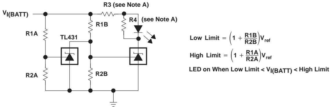
NOTE A: R3 and R4 are selected to provide the desired LED intensity and cathode current  $\geq 1$  mA to the TL431 at the available  $V_{I(BATT)}$ .
