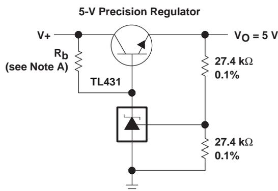
NOTE A: R<sub>b</sub> should provide cathode current ≥ 1 mA to the TL431.
